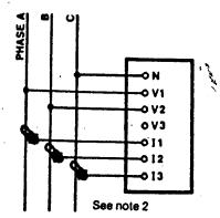
Note 1 - this configuration requires a balanced system. All Voltage readings must be multiplied by 1.73.
