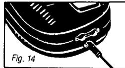
2. Insert ohmmeter battery/fuse attachment into the jack on the right side of the instrument just below the ohmmeter Zero Adjust Knob. Seat plug to bottom for good connection (Fig. 15).
